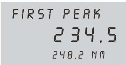
Display in "First Peak" mode showing torque readings
